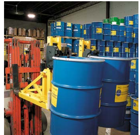
Double gripping heads are best for light gauge open head drums
