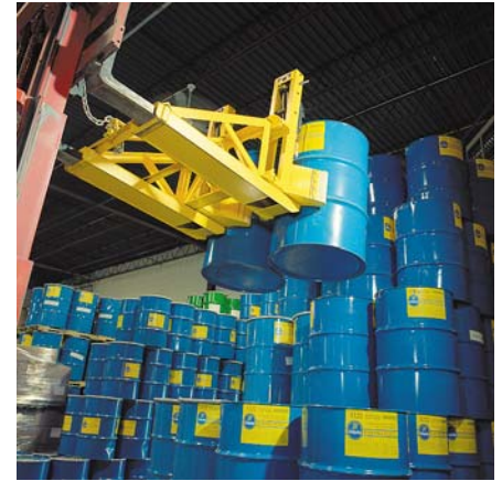
Step tiering drums without pallets saves valuable warehouse space
