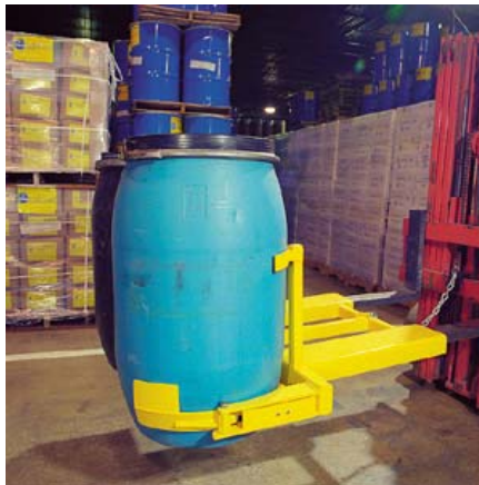
Drums rest against circular backrest for vertical support
